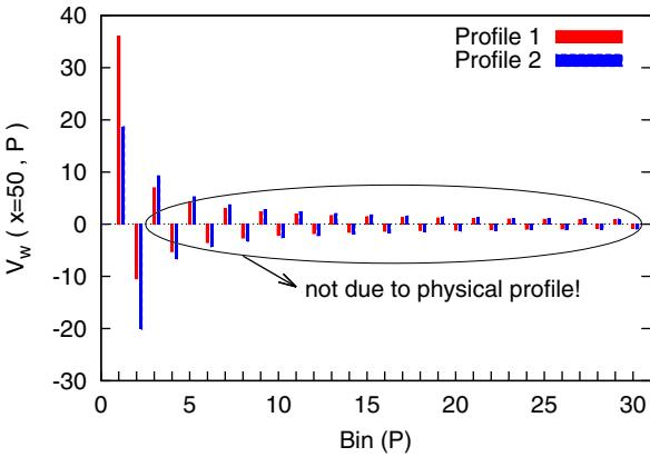
Fig. 2. Wigner potential at a fixed position,  $V_W(x = 50, P)$ , for the profiles in Fig. 1, calculated with a coherence length of  $\mathbf{L} = \mathbf{L}_{dev}$ .
