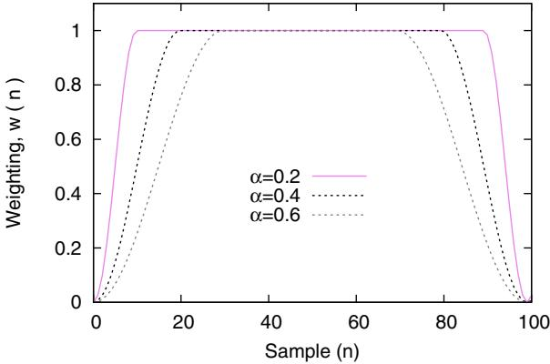
Fig. 3. Tukey window function, for various values of  $\alpha$ , used to smooth the potential values toward zero at the boundaries by appropriately weighting the samples (potential difference values) used to compute the DFT in the Wigner potential.
