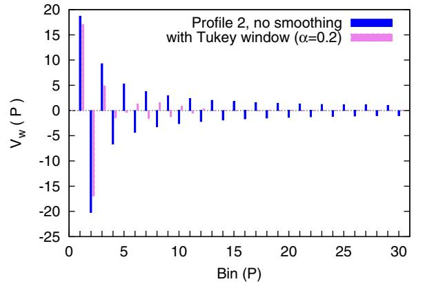
Fig. 4. The unnormalized Wigner potential,  $V_W(x = 50, P)$ , calculated at the centre of the device with and without the application of a smoothing Tukey window ( $\alpha = 0.2$ ), using Profile 2 (blue) in Fig. 1, and a coherence length of  $\mathbf{L} = \mathbf{L}_{dev}$ .
