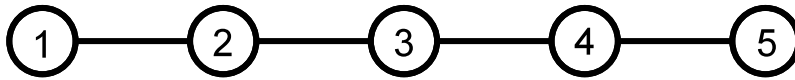
Figure 1.1: Graph representation of the discretization of equation 1.1. Numbered circles denote points, lines symmetric connections between points.
