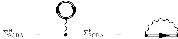
Figure 3.9: FEYNMAN diagrams of the self-consistent first-order proper self-energies.
