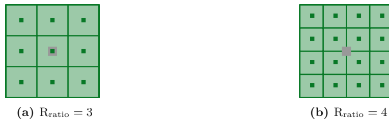
Figure 6.3: Illustration of a grid point with two refined grids with different refinement ratios R_{\text{ratio}} .
