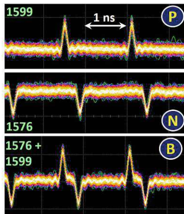
Figure 2.21: Simultaneous reception of weighted spike trains summed by the synaptic receptor (B) where the constituent wavelength channels at 1576 nm and 1599 nm are weighted negatively (N) and positively (P), respectively [MVS1], [MVS3].
