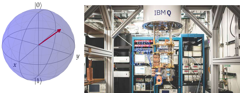
Figure 1.2. Left: Mathematical representation of a qubit as Bloch sphere, which represents all possible states as superposition of \alpha |0\rangle + \beta |1\rangle . Operations on a qubit are represented by unitary matrices, resulting in a rotation of the vector on the sphere. Right: Quantum computer from the IBM Q project. The golden chandelier in the photograph shows different stages, from the mK-stage at the bottom to room temperature at the top. Figure taken from [60].
