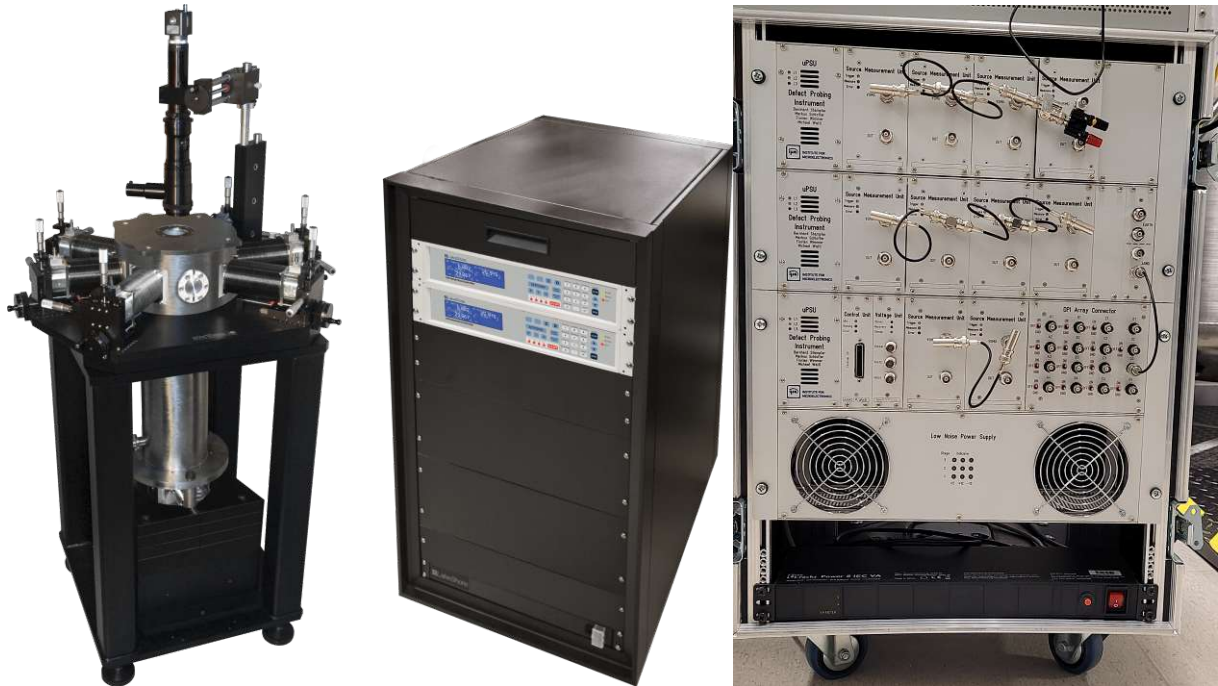
Figure 5.1. A LakeShare CPX-4K cryogenic probe station (left) was used for time-zero and reliability characterization of various technologies. A custom built measurement box with ten SMUs (right) was used for the characterization of transistor arrays. Left two images courtesy Lake Shore Cryotronics, Inc.
